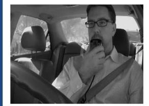
A camera eliminates the excuse that the interlock violation was by another person. It also ensures the offender is the one using the device. The camera is safely mounted near the dashboard.
